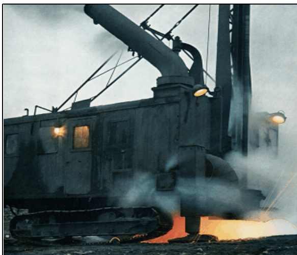
Fig. 12. Modern machinery for extracting iron from poor ores, by melting them under electric arc (2500°C)
