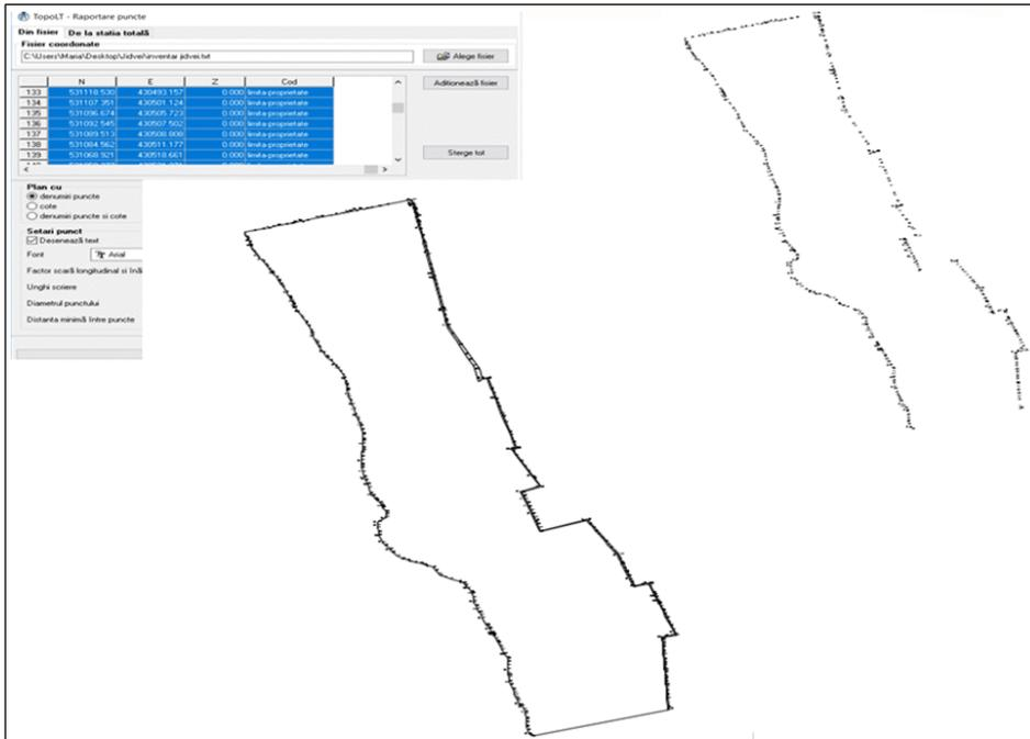
Fig. 6. The imports of the points coordinates and the representation of the measured objective
