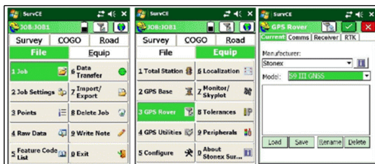
Fig. 3. Connecting the receiver to the GPS station 7
