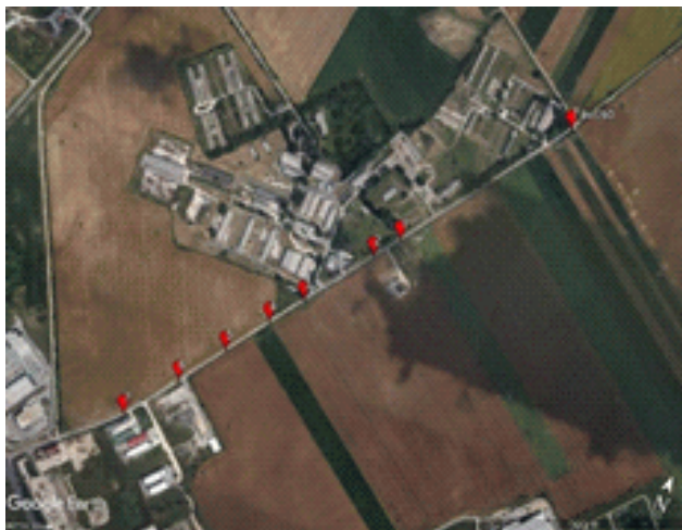
Fig. 5. Telescopic measurement: positions of the telescope placed during the measurement and of the measuring rod set up during taking each photograph
