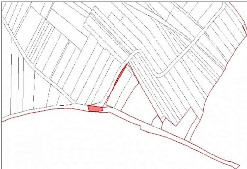
Fig. 2. Gaps and overlaps in the cadastral plan, when checking the topology
