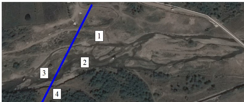
Fig. 4. The state of the bed of the Tazlaul Sarat River in the research area after the flood: 1 – old bed; 2 – new bed created during the flood; 3 – the undercrossing area; 4 –adduction pipe (Google earth image 2017)
