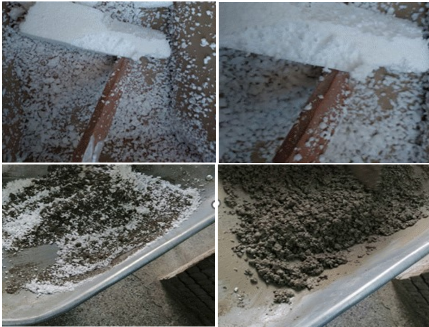
Figure 2. EPS shredding and mixing (Source: Own processing)
