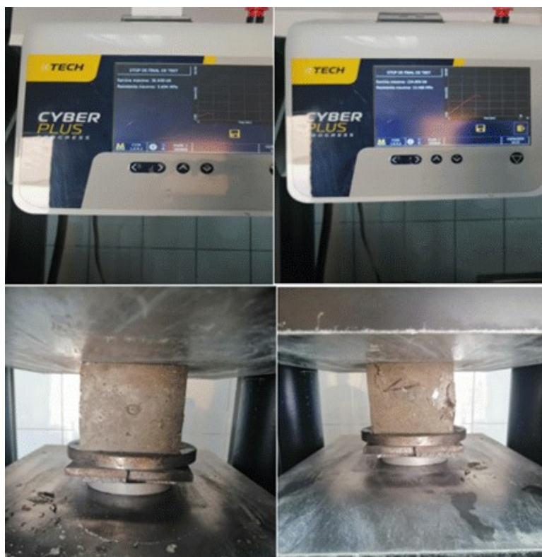
Figure 4. Carrying out compressive strength tests (Source: Own processing)
