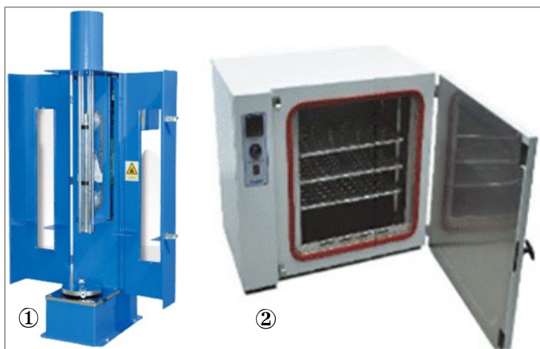
Fig. 3: 1- Proctor UTS-0620 automatic compactor (18) 2 - Ventilated oven with thermostat UTD-1295 (19)
