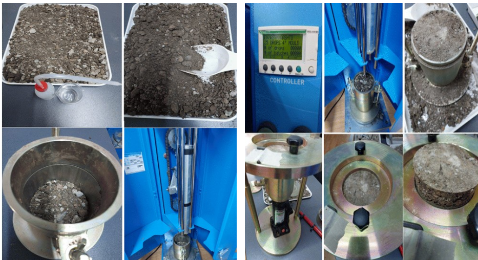
Fig. 5. Stages of the normal Proctor trial
