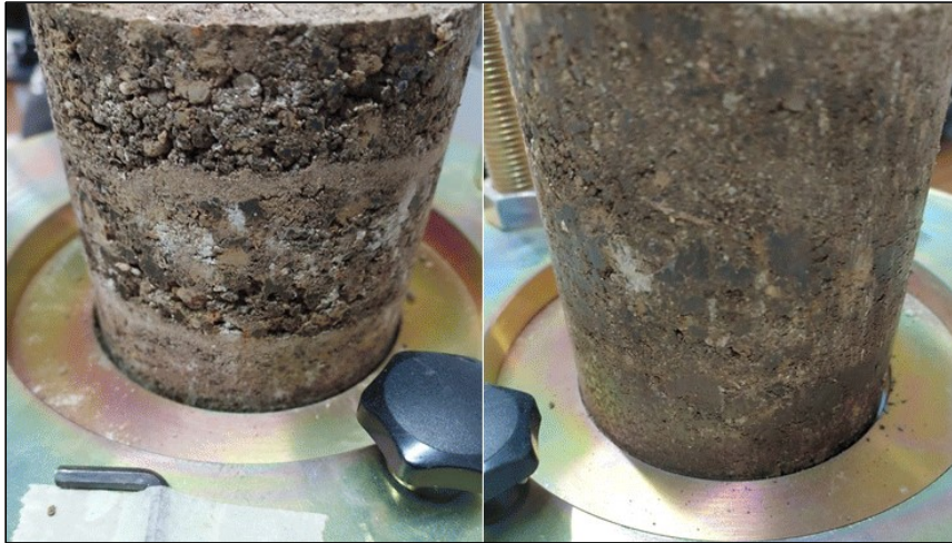
Figure 7. The differences between the initial material compacted with natural moisture and the material compacted with the addition of water
