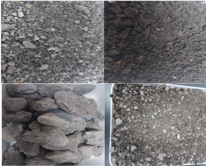
Fig. 4. Material samples subjected to the normal Proctor test
