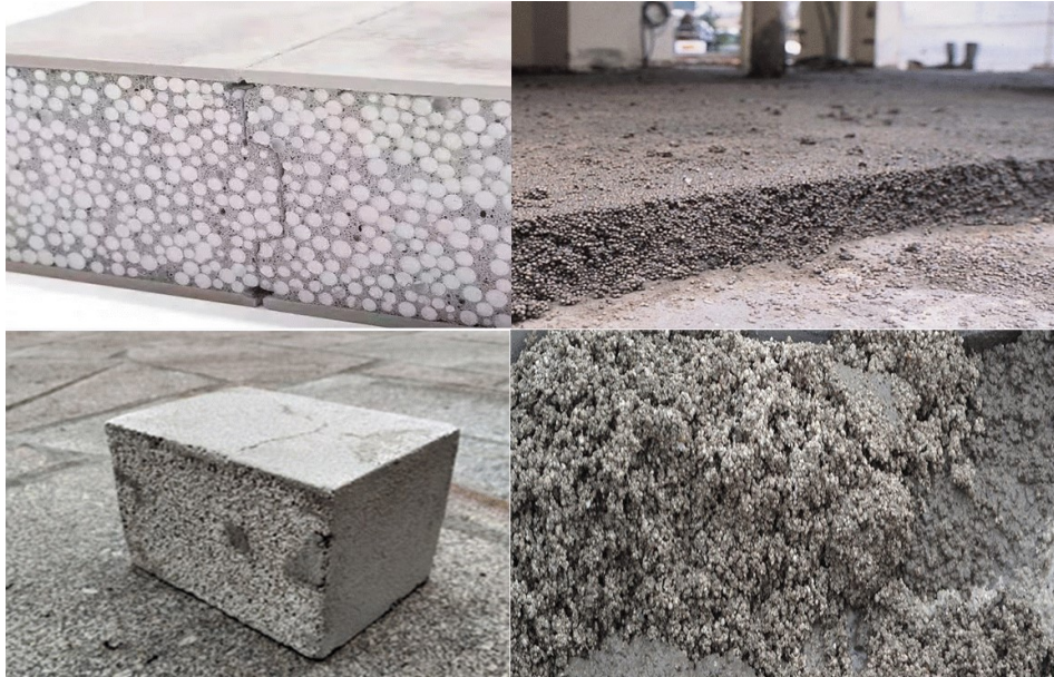
Fig. 3. Uses of concrete with polystyrene (18–21)
