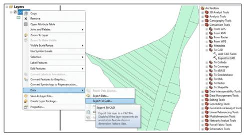
Fig.8. DWG / DXF export possibilities - layer and multilayer
