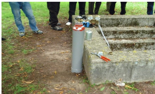
Fig. 3. Preparation and injecting tracer gas
